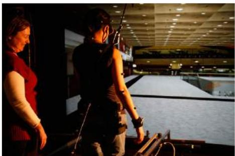
Figure 4. Self-paced treadmill locomotion in a complex VE (CSM)
